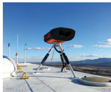
Lidar sensor on a nacelle: Wind Iris from Avent Lidar Technology.
